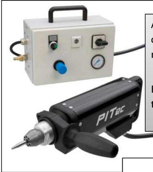
An artificial muscle, a new development of **FESTO**, is driven by way of compressed air. These motions are transferred as hammering movements on one or more pins.
