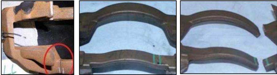
➤ Crack in the prototype – Brake Carrier after 2/3 of the required fatigue life.
