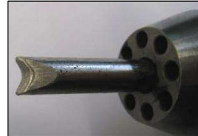
PIT treatment of the stress hotspots by way of a concave pin.
