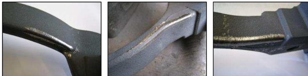
Fatigue life enhancement of 11 times compared to the untreated Brake Carrier
